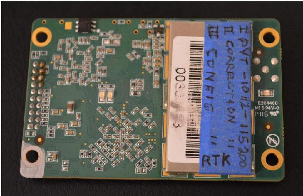
K501G with port function and baud rate labeled on blue tape
